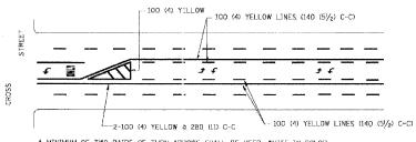
A MINIMUM OF TWO PAIRS OF TURN ARROWS SHALL BE USED, WHITE IN COLOR. ADDITIONAL PAIRS SHALL BE PLACED AT 60 m (200') TO 90 m (300') INTERVALS.
