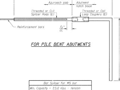
Min. Capacity = 23.0 kips - tension Min. Pull-out Strength = 9.2 kips - tension No. Required = N/A
