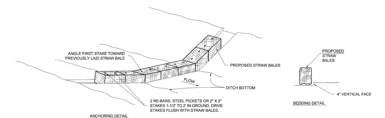
APPROXIMATELY 9 STRAW BALES SHALL BE REQUIRED PER DITCH CHECK "NOT TO SCALE"
