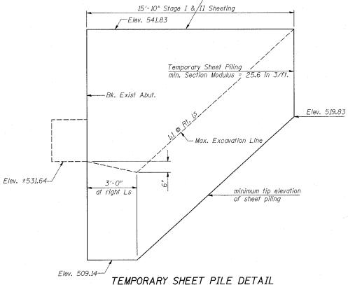
If the Contractor chooses to alter the temporary cantilevered sheet piling design requirements shown on the plans, a design submittal including plan details and calculations will be required for review and acceptance by the Engineer.
