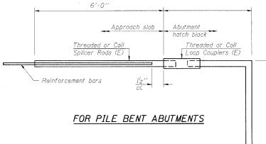
Bar Splicer for #5 bar Min. Capacity = 23.0 kips - tension Min. Pull-out Strength = 9.2 kips - tensio Required =
