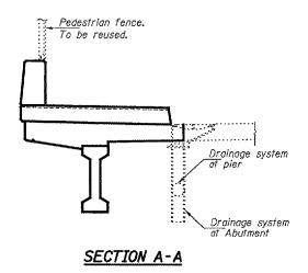
\* The Contractor shall ensure that the scupper is supported at all times during the construction process.
