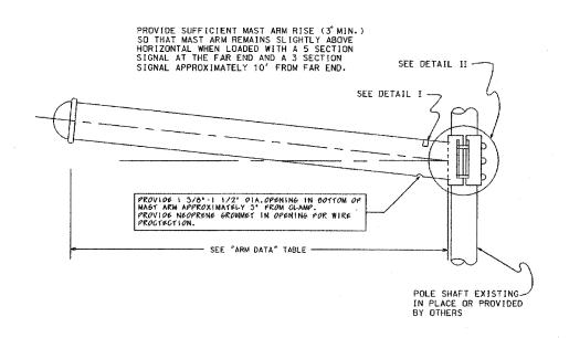
ARM DATA TEST LOAD (POUNDS) (INCHES) SIGNAL END LENGTH (FEET) WEIGHT (POUNDS) MAX. DEFLECTION 7.45-7.95 7.0 4.76 16 241 1700 7.45-7.95 7.0 4,20 274 1300 12.0 7.45-7.95 7.0 3,36 26 315 1000 24.0 8.45-8.95 8.0 3.80 30 409 1100 29.0 9.95-10.45 9.0 4.10 35 529 1200 36.0 9.95-10.45 9.0 3.40 40 559 1000 52.0 9.95-10.45 10.0 3.84 44 1200 57.0
