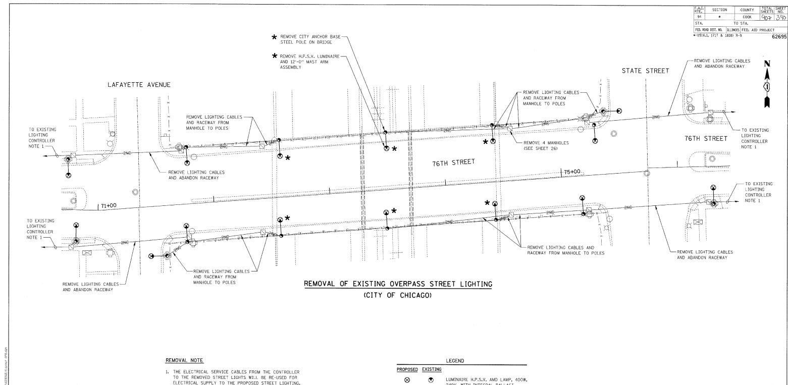
. THE ELECTRICAL SERVICE CABLES FROM THE CONTROLLER TO THE REMOVED STREET LIGHTS WILL BE RE-USED FOR ELECTRICAL SUPPLY TO THE PROPOSED STREET LIGHTING. PROVISIONS SHALL BE MADE AT THE MANHOLES OR LIGHT POLES FOR SPLICING THE EXISTING CABLES FOR THE PROPOSED CABLES TO THE NEW STREET LIGHTING.
