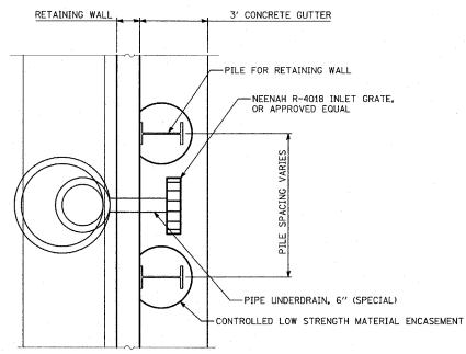
PLAN, CONCRETE GUTTER OUTLET
