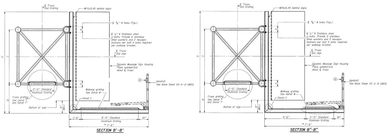
\* Bracket and grating dimensions are nominal and will vary based on actual DMS cabinet dimensions plus manufacturer's mounting devices, and providing clearance between the lowered handrail and DMS cabinet.
