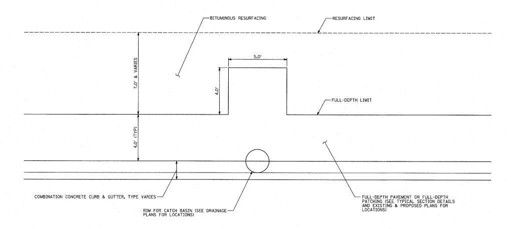
NOTE: LOCATION OF ADDITIONAL PAVEMENT IN RELATION TO CATCH BASIN LOCATION IS DETERMINED BY THE ORIENTATION OF THE EXISTING SEWER UNDER THE FRONTAGE ROAD.
