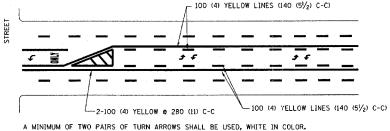
A MINIMUM OF TWO PAIRS OF TURN ARROWS SHALL BE USED, WHITE IN COLOR. ADDITIONAL PAIRS SHALL BE PLACED AT 60 m (200') TO 90 m (300') INTERVALS.
