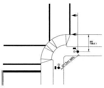
RECOMMENDED PUSHBUTTON LOCATIONS FOR ACCESSIBLE PEDESTRIAN SIGNALS SHALL BE IN ACCORDANCE WITH THE CURRENT MUTCD (SEE NOTE I). TO MEET MUTCD REQUIREMENTS, PEDESTRIAN SIGNAL PUSHBUTTONS MAY HAVE TO BE MOUNTED ON A SEPARATE POST.
