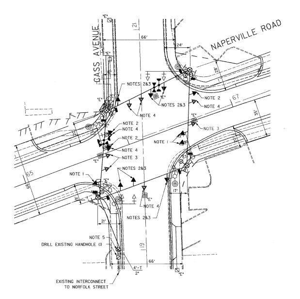
NOTE I: THE SIGNAL HEADS FOR THE EASTBOUND TRAFFIC SHALL BE DISCONNECTED AND BAGGED DURING CONSTRUCTION STAGES PRE-STAGE I, STAGE I, AND STAGE 2, AND SHALL BE ACTIVATED AFTER ALL THE PAVEMENT GEOMETRICS ARE IN PLACE AND TWO-WAY TRAFFIC MOVEMENT IS ALLOWED PRIOR TO ACTIVATION OF THE NEW PERMANENT SIGNALS. THE CONTRACTOR CAN, HOWEVER, INSTALL THESE SIGNAL HEADS PRIOR TO COMPLETION OF STAGE 2 CONSTRUCTION AS DIRECTED BY THE ENGINEER.
