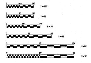
FULL SIZE PLANS HAVE BEEN PREPARED USING STANDARD ENGINEERING SCALES, REDUCED SIZED PLANS WILL NOT CONFORM TO STANDARD SCALES, IN MAKING MEASUREMENTS ON REDUCED SIZED PLANS, THE ABOVE SCALES MAY BE UTILIZED.
