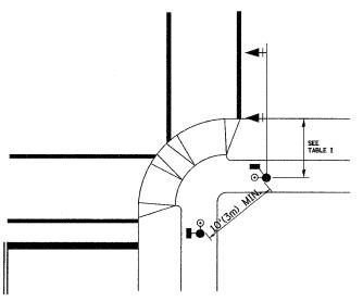
RECOMMENDED PUSHBUTTON LOCATIONS FOR ACCESSIBLE PEDESTRIAN SIGNALS SHALL BE IN ACCORDANCE WITH THE CURRENT MUTCD (SEE NOTE 1). TO MEET MUTCD REQUIREMENTS, PEDESTRIAN SIGNAL PUSHBUTTONS MAY HAVE TO BE MOUNTED ON A SEPARATE POST.
