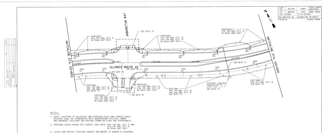
4. PROPOSED 100mm PUSHED GRS CONDUIT (32m) WITH: 2\*4, 1\*8 GND. (CCT 3) AND 2\*4, 1\*8 GND. (CCT 4) IN 50mm UNIT DUCT
