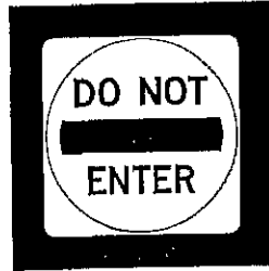
(E) 48" X 48" Std. 36" X 36" R5-1 or 36" X 36" overall with Std 36" X 36" R5-1 where noted
