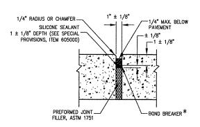
\* POLYETHYLENE OR POLYESTER TAPE (3 MIL. MIN.) OR MARKING TAPE, RUBBER TAPE, 1/8" WIDER THAN WIDTH OF JOINT.
