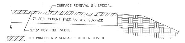
NOTE: SQUARE YARDAGE OF SURFACE REMOVAL WAS CALCULATED USING THE WIDTH OF THE PROPOSED SURFACE, ANY ADDITIONAL REMOVAL NEEDED FOR PROPER OPERATION OF PAVING EQUIPMENT WILL BE THE CONTRACTORS RESPONSIBILITY AND NO ADDITIONAL COMPENSATION WILL BE ALLOWED.
