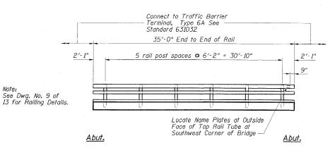
RAILING ELEVATION (Showing Inside Face of North Railing; South Railing Similar)
