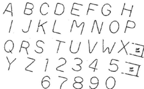
Figure 4-2-2. Design of Special Letters and Numbers on a 10 Degree Angle for Rail Stamps, No Sharp Corners
