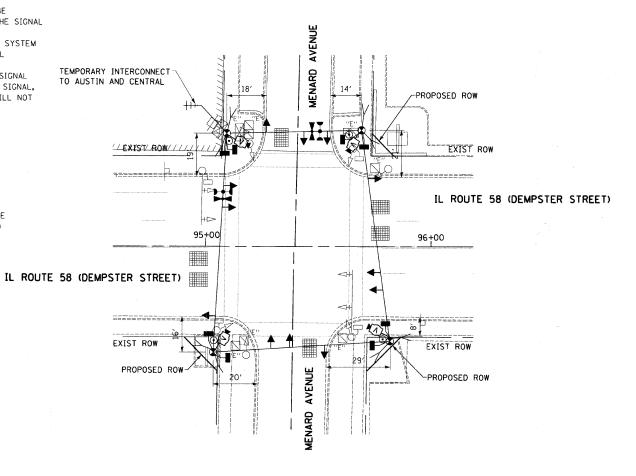
THE FOLLOWING ITEMS SHALL BE REMOVED BY THE CONTRACTOR AND SHALL BE DISPOSED OF BY THEM OUTSIDE OF THE RIGHT-OF-WAY AT THEIR EXPENSE, THE SALVAGE VALUE OF THE REMOVED EQUIPMENT SHALL BE REFLECTED IN THE CONTRACT BID PRICE.
