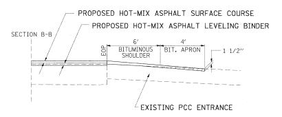
PREPARATION OF EXISTING SURFACE AND ANY EXCAVATION FOR ENTRANCES SHALL BE IN ACCORDANCE WITH ARTICLE 406.09 OF THE STANDARD SPECIFICATIONS.
