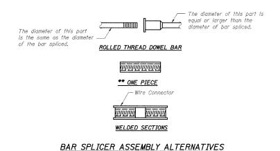
\*\* Heavy Hex Nuts conforming to ASTM A 563, Grade C, D or DH may be used.
