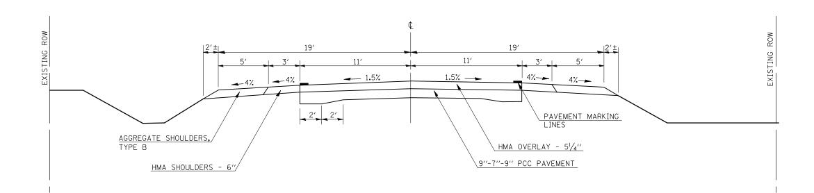
NOTE: SHOULDERS ARE A BAM MIX AND WILL NEED TO BE MILLED SEPARATELY FROM MAINLINE PAVEMENT SO THAT RAP CAN BE STOCKPILED SEPARATELY.
