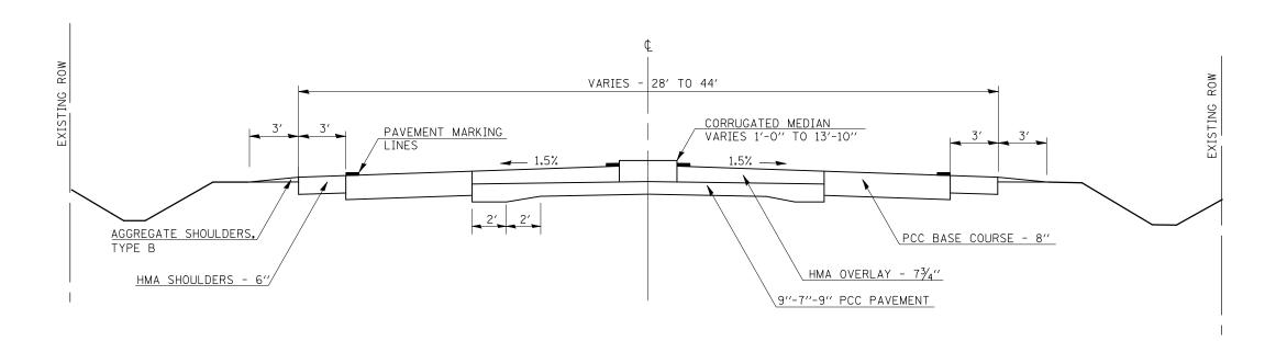
NOTE: SHOULDERS ARE A BAM MIX AND WILL NEED TO BE MILLED SEPARATELY FROM MAINLINE PAVEMENT SO THAT RAP CAN BE STOCKPILED SEPARATELY.
