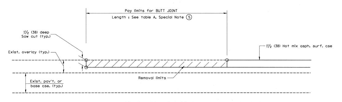
CASE 5: WITH HOT MIX ASPHALT SURFACE REMOVAL (COLD MILLING)
