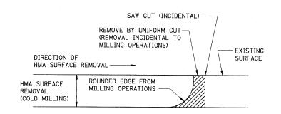
NOTE: WHEN MILLING OPERATIONS PRODUCE A ROUNDED EDGE, THEN A SAW CUT SHALL BE USED TO MANUFACTURE A PERPENDICULAR EDGE AS SHOWN IN THE DETAIL. THE ENGINEER SHALL BE THE SOLE JUDGE CONCERNING THE USE OF THIS DETAIL.
