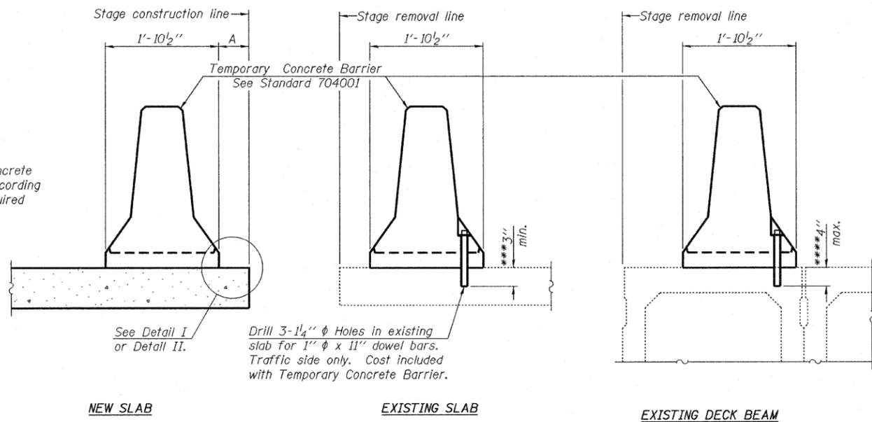
Drill 3-1/4"  $\phi$  Holes in existing slab for 1"  $\phi$  x 11" dowel bars. Traffic side only. Cost included with Temporary Concrete Barrier.
