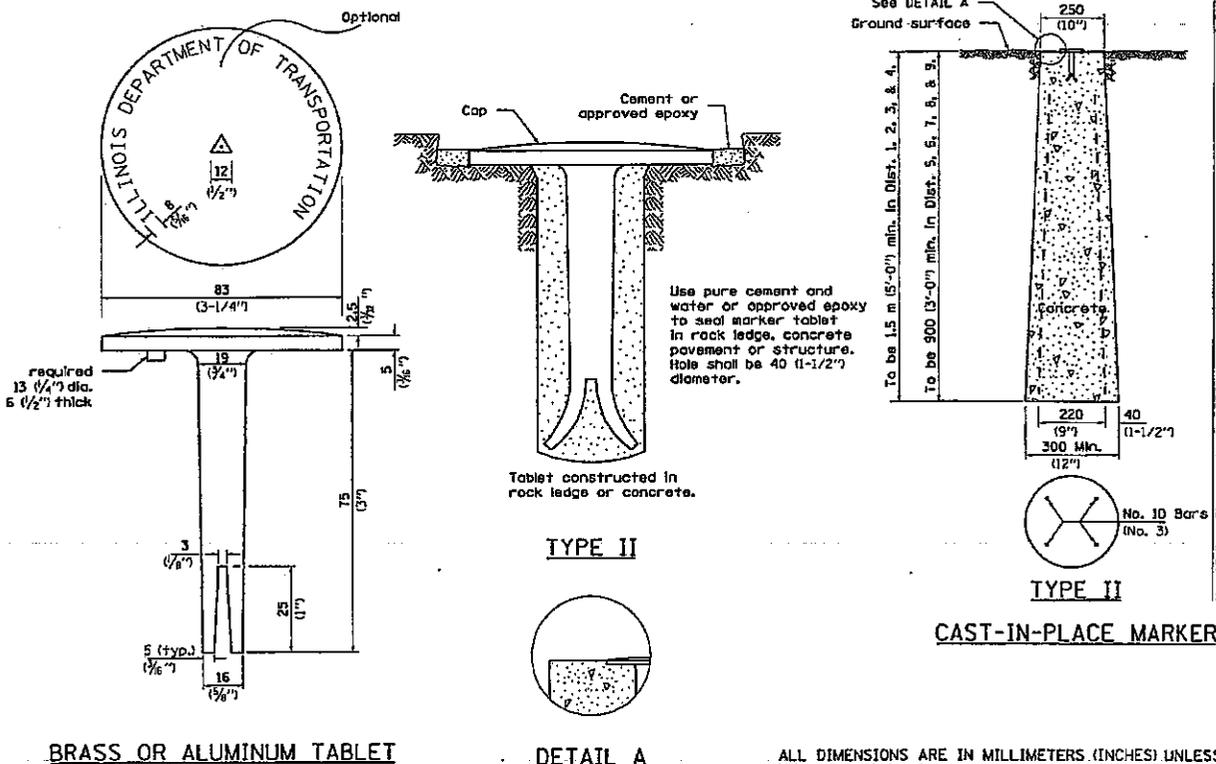
No. 10 (No. 3) bars to be 750 (30") for 900 (35") min. & 1.1 m (3'-6") for 1.2 m (4'-0") min.
