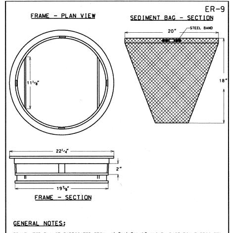
FRAME: TOP FLANGE FABRICATED FROM 114"X114"X1/8" ANGLE. BASE RIM FABRICATED FROM 11/2"X1/2"X1/8" CHANNEL. HANDLES AND SUSPENSION BRACKETS FABRICATED FROM 11/4"X1/4" FLAT STOCK. ALL STEEL CONFORMING TO ASTM-A36. SEDIMENT BAG: BAG FABRICATED FROM 4 OZ./ SQ.YD. NON-WOVEN POLYPROPYLENE GEOTEXTILE REINFORCED WITH POLYESTER MESH. BAG SECURED TO BASE RIM WITH A STAINLESS STEEL STRAP AND LOCK. FILTER FOR OTHER SHAPE GRATES SHALL BE APPROVED IN ADVANCE OF PLACEMENT
