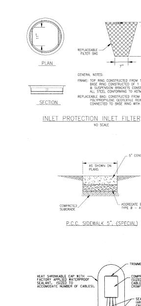
TRIMMED CABLES HEAT SHRINKABLE CAP WITH FACTORY APPLIED WATERPROOF SEALANT. (SIZED TO ACCOMODATE NUMBER OF CABLES). COMPRESSION TYPE COPPER SLEEVE. (SIZED FOR ACTUAL NUMBER OF CABLES AND MFR. SUGGESTED CRIMP TOOL USED). - SEALANT TAPE OR INSERT. (AROUND AND THROUGH CROTCH OF SPLICE). ELECTRIC FEEDER CABLES, (SIZE AS NOTED ON CONTRACT DRAWINGS). NOTE: NUMBER OF CABLES IN SPLICE MAY VARY SPLICING ELECTRICAL CABLES
