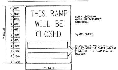
THESE SIGNS ARE REQUIRED ON BOTH SIDES OF THE RAMP, MINIMUM OF I WEEK IN ADVANCE OF THE CLOSURE.
