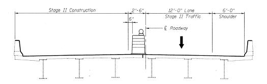
STAGE 2 CROSS SECTION (LOOKING NORTH) PROPOSED CONSTRUCTION STAGING
