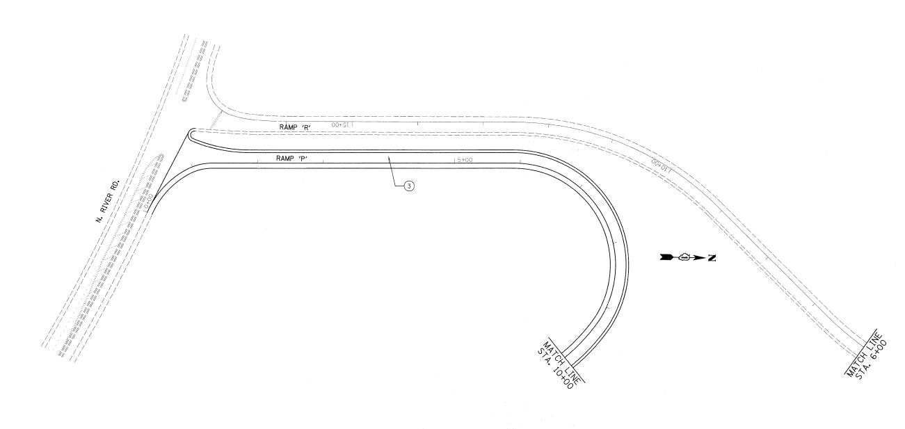
1)—— PROP. HOT-MIX ASPHALT SURFACE REMOVAL, 4"
