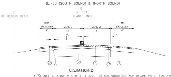
\*(3) MILL 4" LANE 2 & MILL 3 3/4 " OUTER SHOULDER AND PLACE POLY. SMA BINDER COURSE 2" ON LANE 2 AND HMA BINDER COURSE, N70, 2 1/4" ON OUTER SHOULDER
