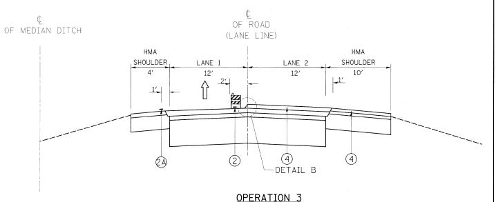
(4) PLACE POLY. SMA SURFACE COURSE 2" ON LANE 2 AND HMA SURFACE COURSE, MIX "D" 1 1/2" ON OUTER SHOULDER
