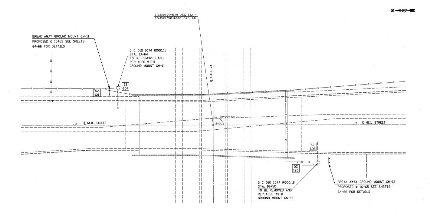
SEE GENERAL NOTE AND SPECIAL PROVISION FOR UTILITY LOCATES. LIGHTING CIRCUIT ELECTRICAL INFO IS APPROX. NO OTHER UTILITIES SHOWN. THE CITY OF CHAMPAIGN IS A JULIE MEMBER AND SHOULD BE CONTACTED TO LOCATE THE TRAFFIC SIGNAL CABLE, LOOPS, AND FIBER OPTIC. CONTRACTOR SHALL VERIFY THIS LOCATE IS DONE PRIOR TO CONSTRUCTION.
