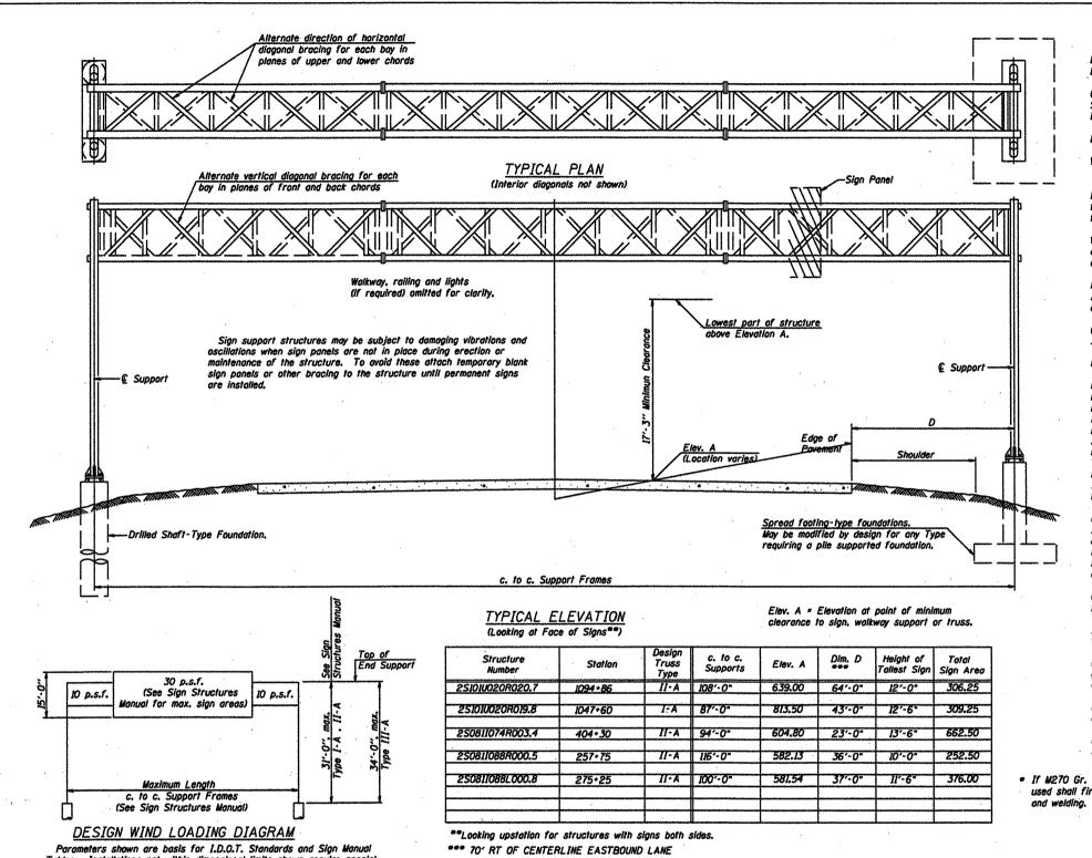
Parameters shown are basis for I.D.O.T. Standards and Sign Manual Tables. Installations not within dimensional limits shown require special analysis for all components.
