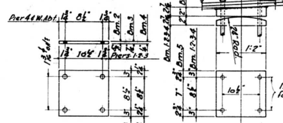
BEARING PLATES AT PIER 2
