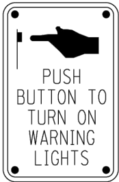
PEDESTRIAN PUSH-BUTTON SIGN DETAILS
