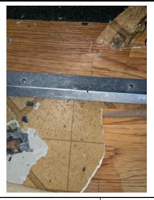
**Material Description:** Tan Linoleum - Tested **Positive for Asbestos**
