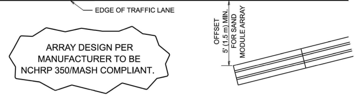
DETAIL "A" IMPACT ATTENUATOR, TEMPORARY (SEE NOTE 5)
