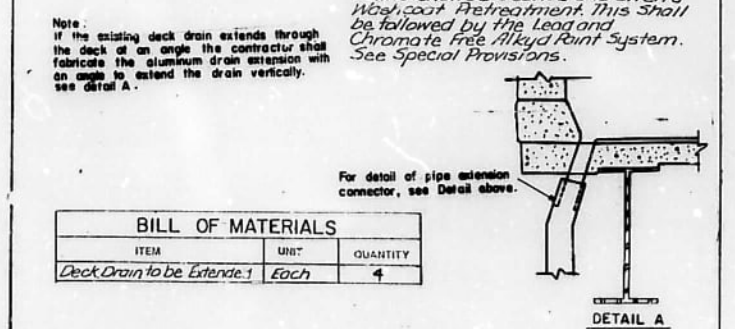
DETAIL OF DECK DRAIN EXTENSION
