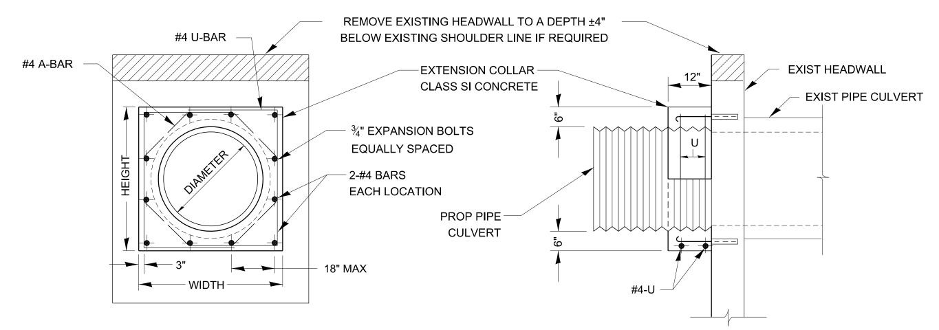
EXPANSION BOLTS SHALL CONSIST OF SELF DRILLING EXPANSION SHIELDS AND <sup>3</sup>/<sub>4</sub>" DIA HOOKED BOLTS. HOOKED BOLTS SHALL EXTEND A MINIMUM OF 9" INTO NEW CONCRETE.
