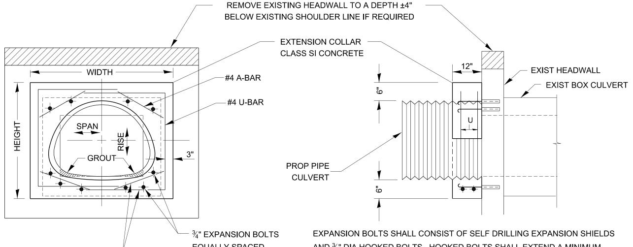
QUANTITIES ARE FOR ONE SIDE ONLY CLASS SI REINFORCEMENT 3⁄4" DIA CONC BARS **EXPANSION** COLLAR BOLTS CU YD POUND EACH
