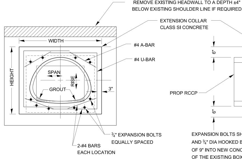
EXPANSION BOLTS SHALL CONSIST OF SELF DRILLING EXPANSION SHIELDS AND <sup>3</sup>/<sub>4</sub>" DIA HOOKED BOLTS. HOOKED BOLTS SHALL EXTEND A MINIMUM OF 9" INTO NEW CONCRETE. BOLTS SHALL BE DRILLED IN THE CENTER OF THE EXISTING BOX CULVERT BARREL WALLS. MINIMUM CERTIFIRED PROOF LOAD = 4,080 LBS.
