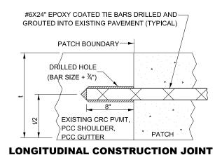
PATCHES MORE THAN 20' IN LENGTH SHALL BE TIED TO ADJACENT PAVEMENT, PCC SHOULDERS OR PCC CURB AND GUTTER WITH #6x24" EPOXY COATED TIE BARS AT 36" CENTERS.
