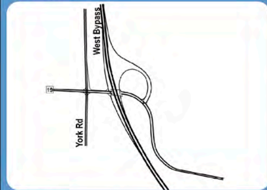
Modified diamond interchange with single loop ramp
