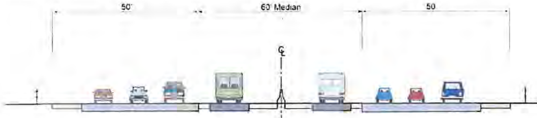
Figure 3 Representative Transit Cross-section without Station West of Meacham Road/Medinah Road (60' Median) a
